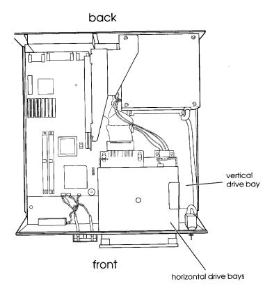
The upper horizontal bay contains the diskette drive that came with your system. If your system came with only one diskette drive, you can install an additional device of one of the following types in the lower horizontal drive bay:
